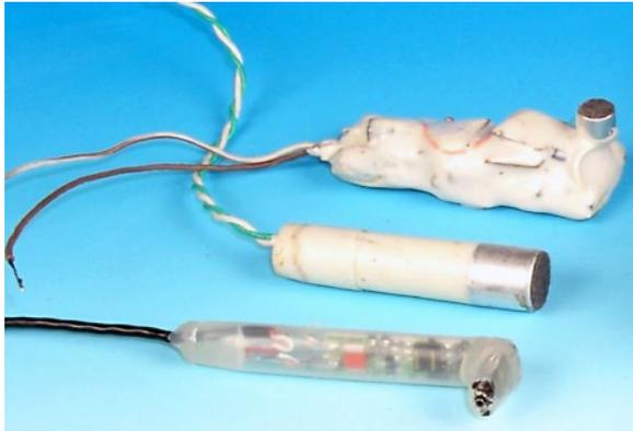
3 generations of Audio Frequency line based NF-B bugs. The 33406-111 bug in the foreground could be fitted in a 10 mm tube.
