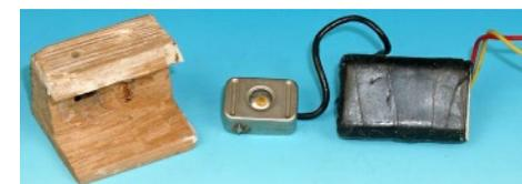
Unknown NF-B bug, with a separate Sennheiser microphone, used in the Rumelsburg prison. The microphone was hidden in a wooden dowel above the cell door.
